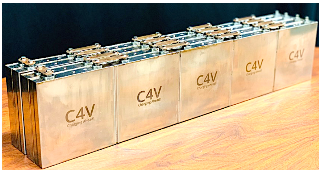
Battery pack designed for MARTAC by C4V team for Autonomous vehicle applications.
