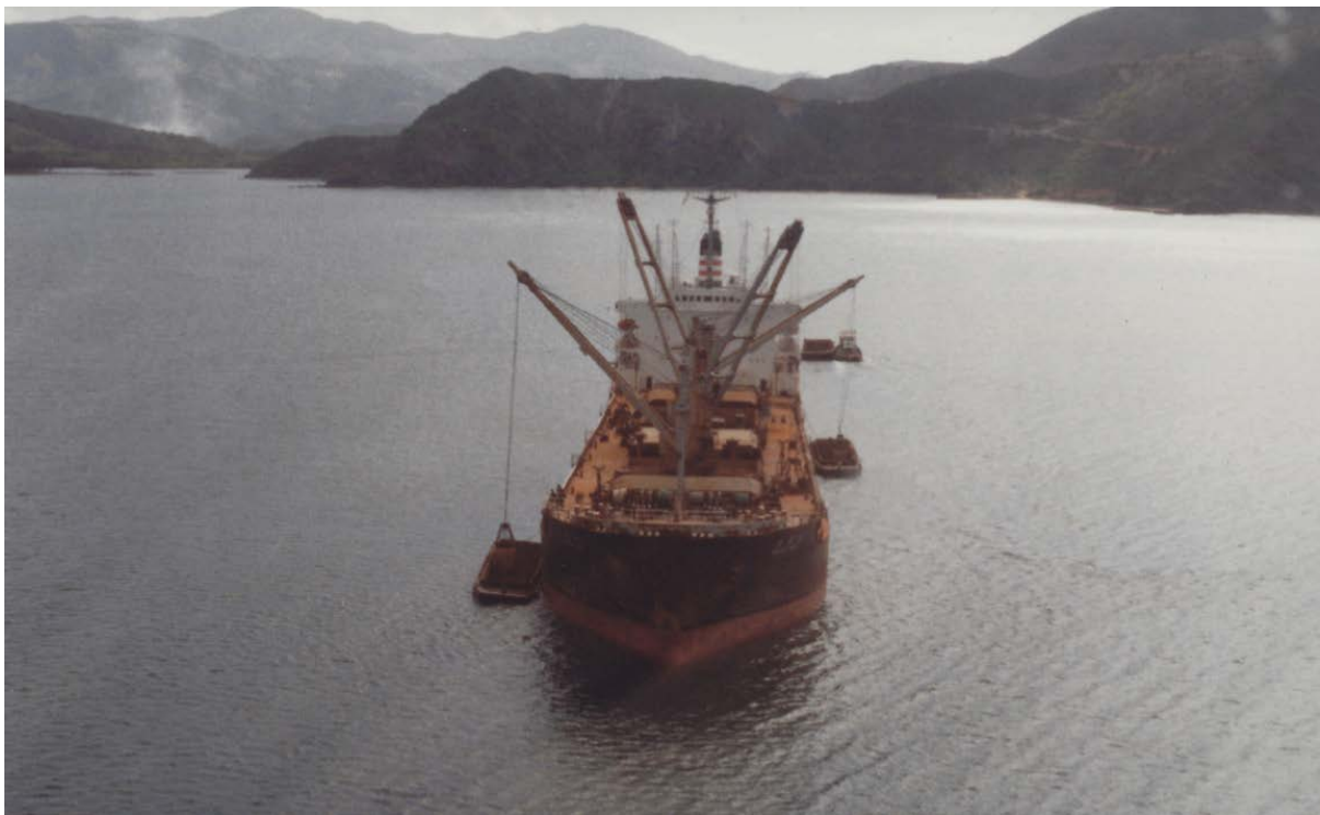
Figure 4: Typical ship loading operations using ships gear
