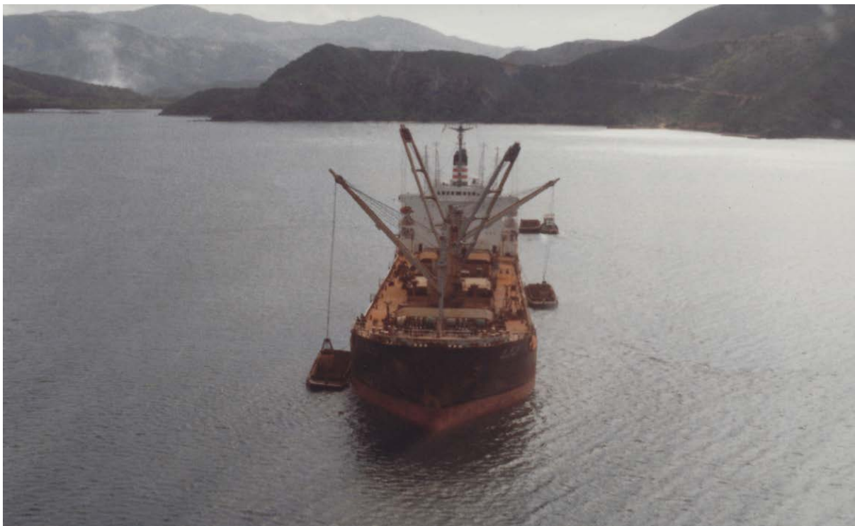
Figure 4: Typical ship loading operations using ships gear
