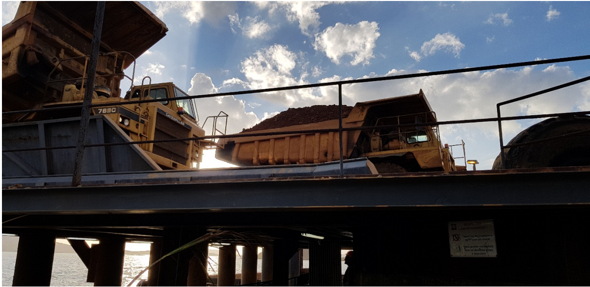
Figure 3: Direct dumping to 300t barges Tontouta (SMGM)
