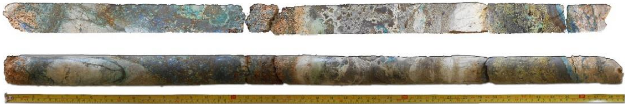
FIGURE 1. Mineralised section of drill core from CMN-3 –136.15-138.10m (1.95m @ 7.72% Cu; 0.11% Co, 0.09% Ni; 0.44% U; 0.24% Zn)
