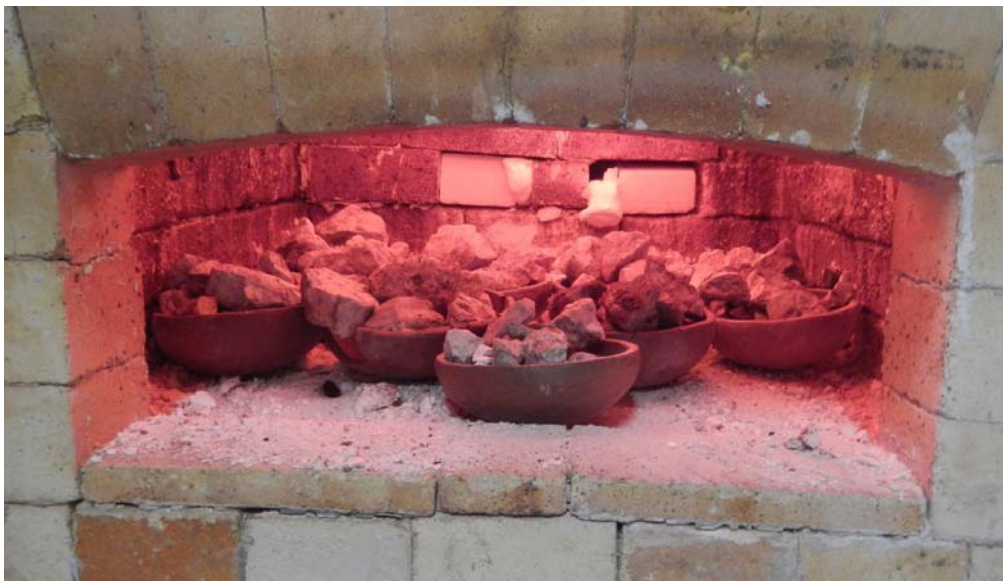
Figure 4 – Decreption Furnace (100kg per day at 1080C)
