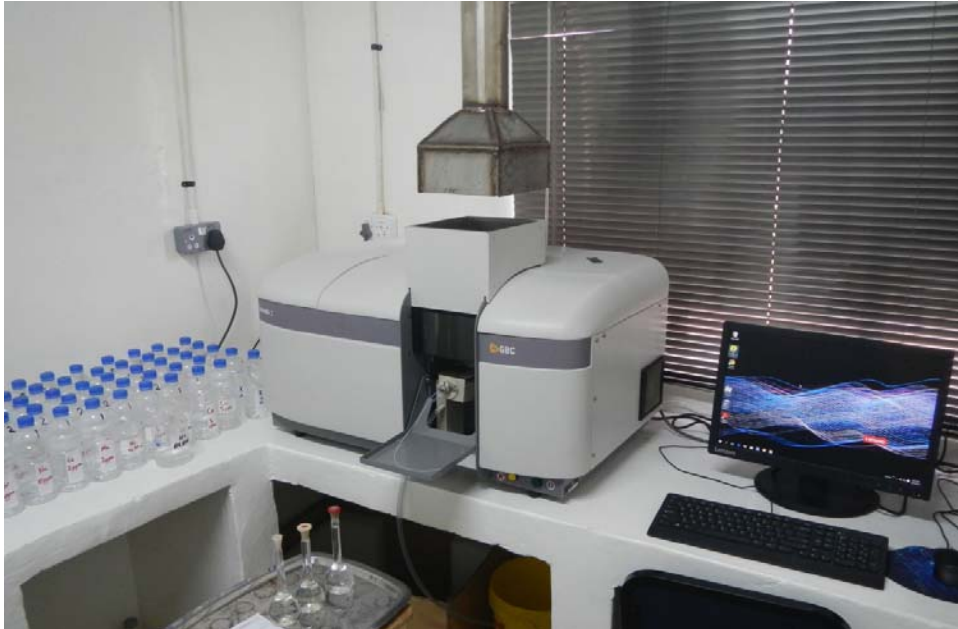
Figure 1 – Atomic Absorption Spectrometer for various elemental analyses
