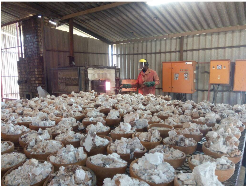
Figure 2 – Pilot Scale Decrepitated Petalite (100 kg per day)
