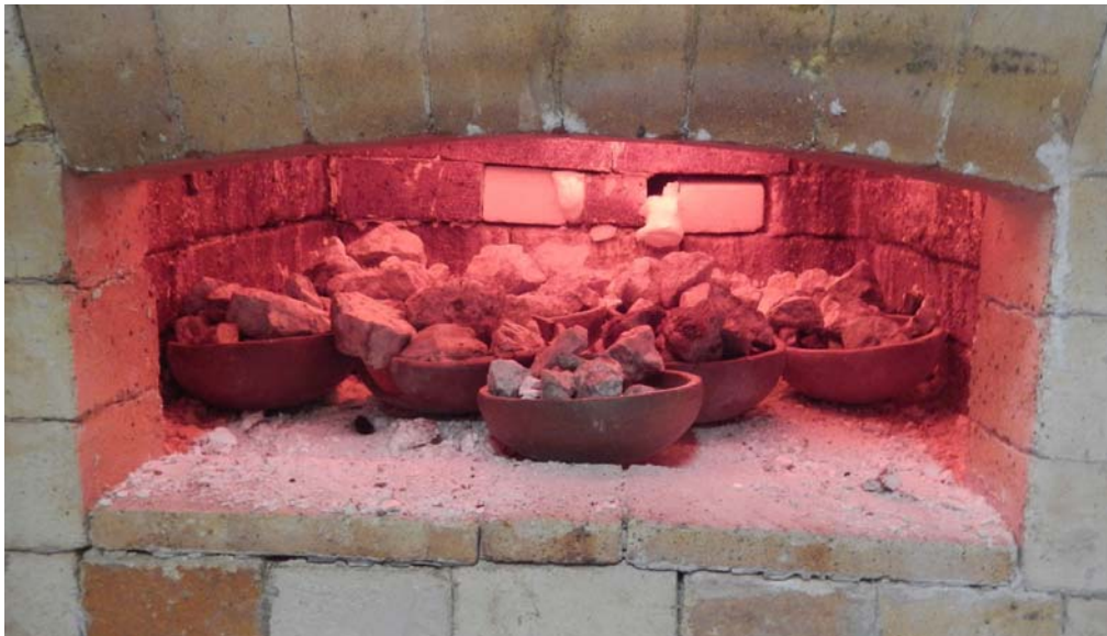
Figure 4 – Decreption Furnace (100kg per day at 1080C)
