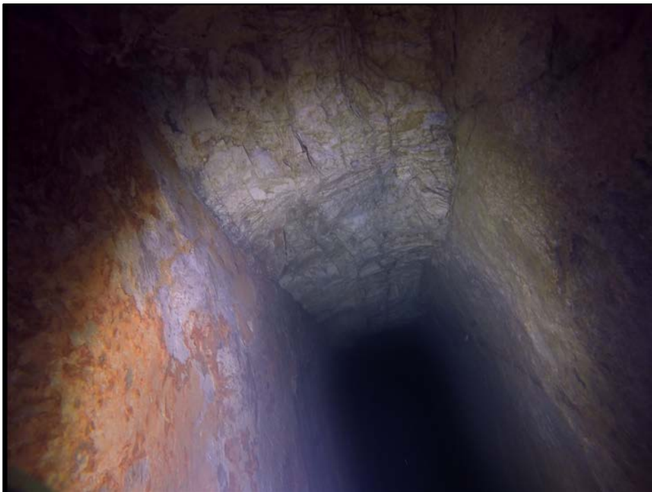
Figure 5: Main Vein exposed in crown pillar of the Level 1 stopes (width approximately 0.75m wide)
