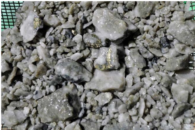
Silicified dacite with chalcopyrite, galena and sphalerite in quartz veining
