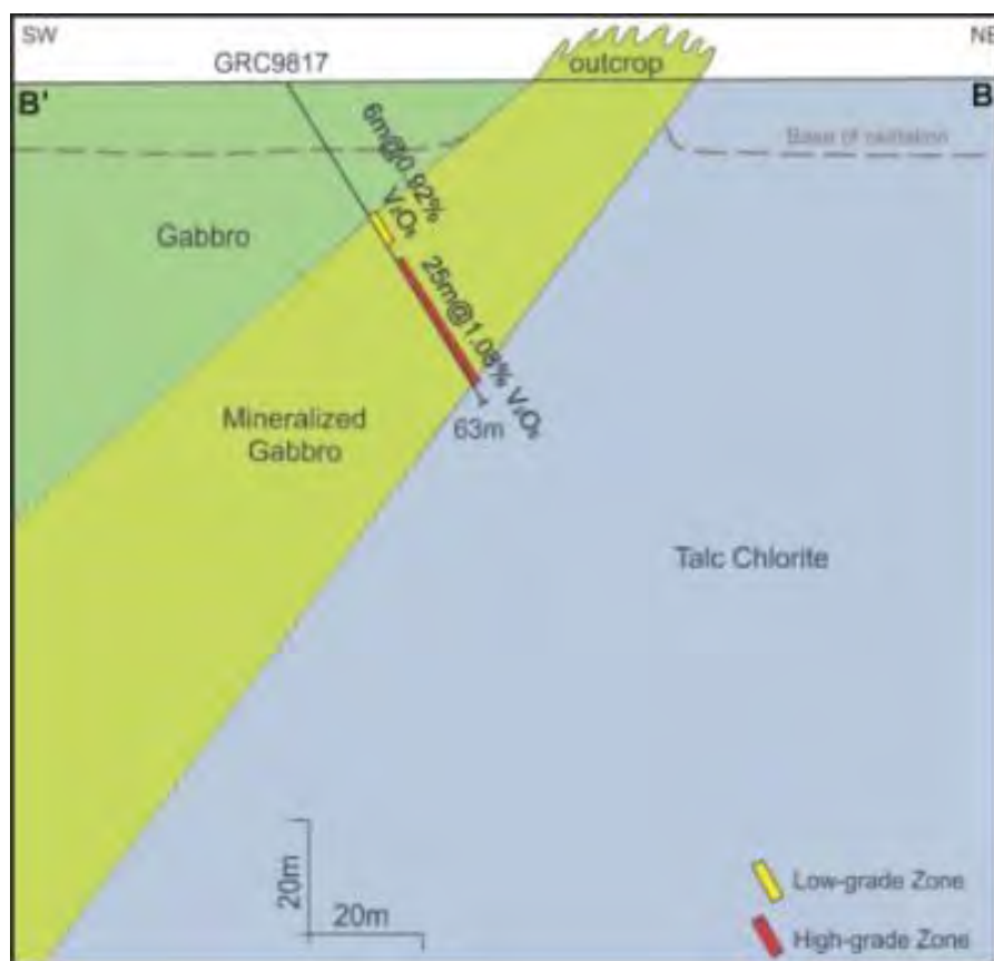
Figure 11: Cross section through P51/2942 showing GRC9817 Mineralised Intersection. 5
