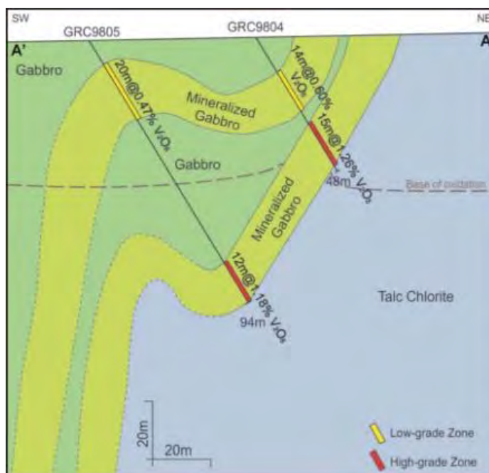
Cross section of previous drilling within Gabanintha Project
