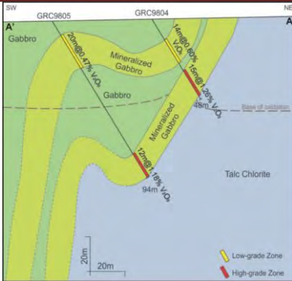
Figure 9: Cross section Through P51/2944 Showing GRC9804 & 5 Mineralised Intersections. 4
