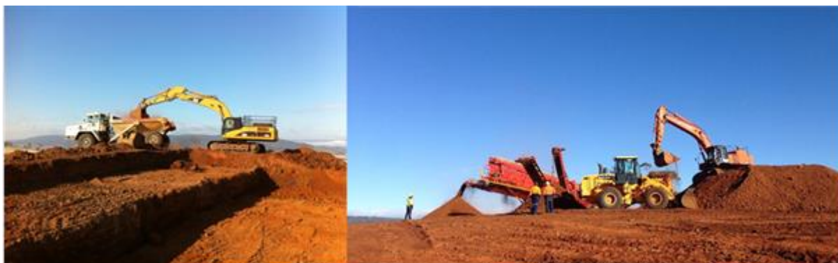
Figures 2 & 3: Bench mining & dry-screening by Stornoway Contractors
