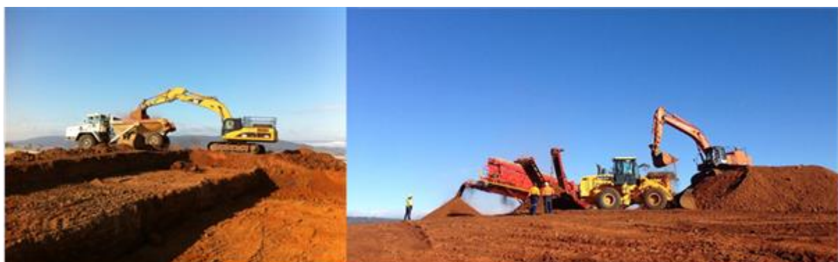
Figures 2 & 3: Bench mining & dry-screening by Stornoway Contractors
