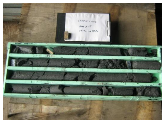
Highly weathered graphitic schist representing the graphite deposit above the base of complete oxidation (BOCO).
