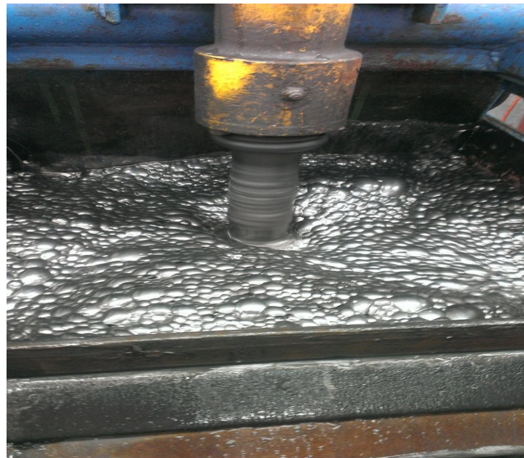
Free flowing well ordered froth conditions during bulk flotation results in less entrainment and excellent launder flow
