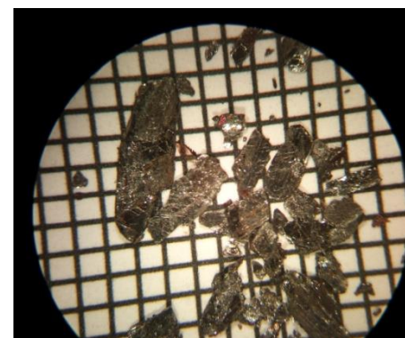
Argent graphite prospect extremely coarse graphite released by knapping a surface rock. Note: the square scale grid is 1 millimeter
