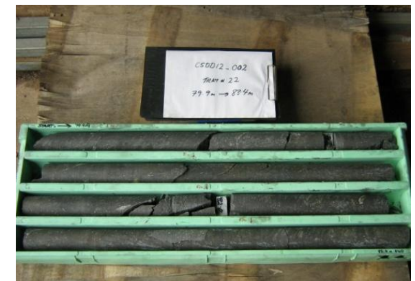
Strongly weathered graphitic schist below BOCO. Graphitic schist progressively more competent with depth.
