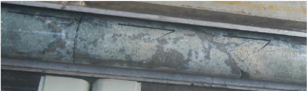
Figure 1: High grade gold mineralisation (silica and sulphide veining) in drill hole TDH08 (122.5m). This example is within a metre sample (122m to 123m) which returned an overall grade of 21.8g/t Au and 19.4g/t Ag.
