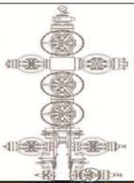
Well Head (3 safety valves)
