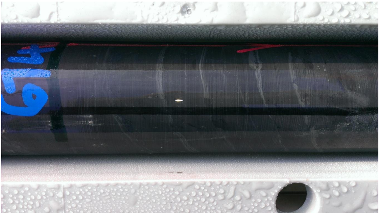
Yallourn Power 1: example from 674 metres of dark grey-black massive shale and thin light grey siltstone laminations with shallow dip.
