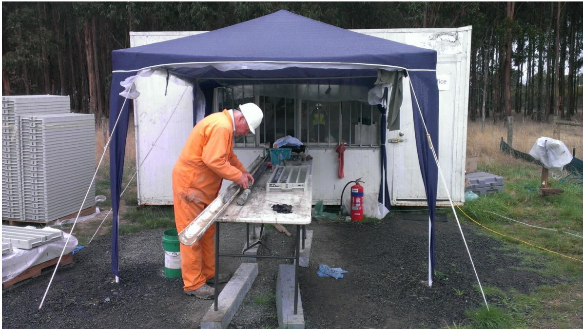
Yallourn Power 1: core tray being marked up on site
