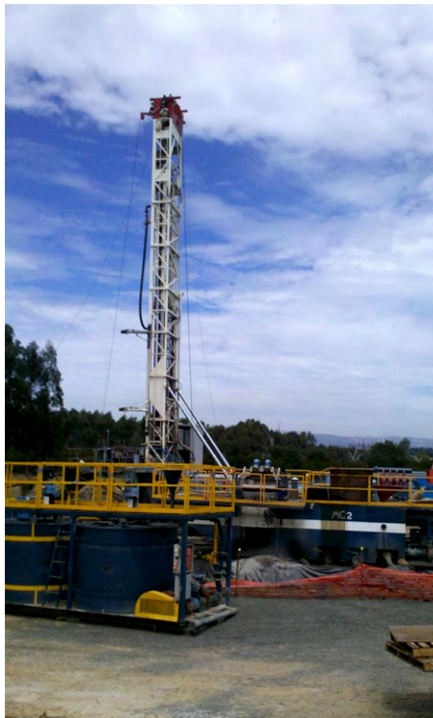
Close up view of Yallourn Power 1 top hole rig (Drilltec Bournedrill TD 2500)
