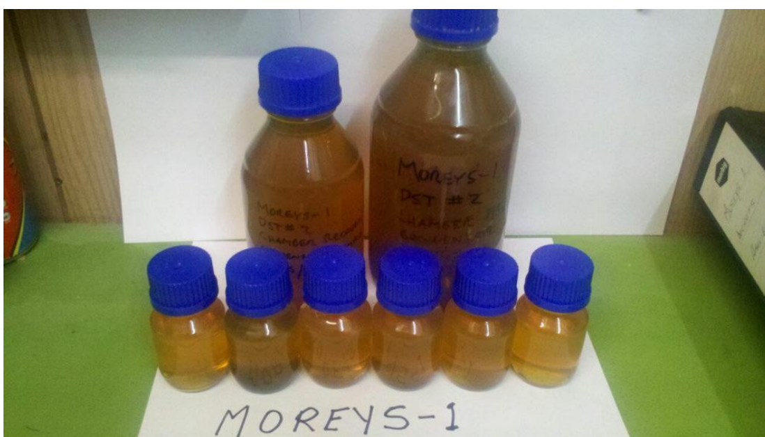
Moreys 1: DST#2 : Condensate collected from Eumeralla Formation
