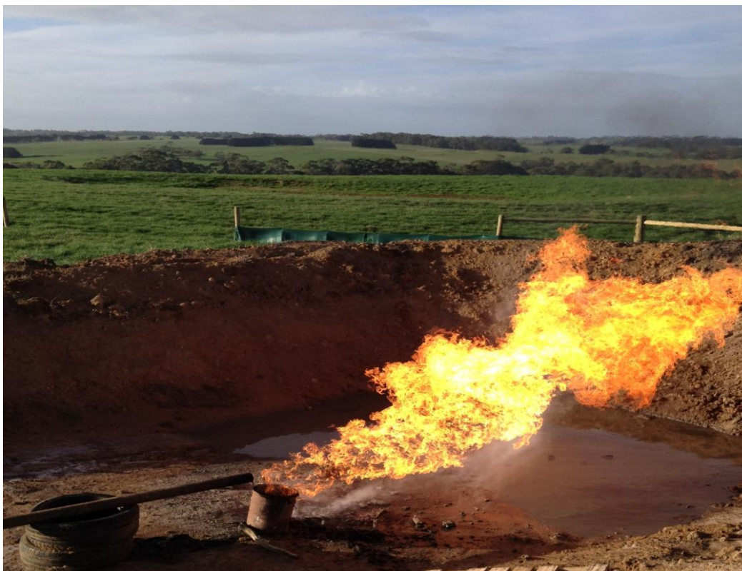
Moreys 1: DST#2: Gas and condensate flare from Eumeralla Formation
