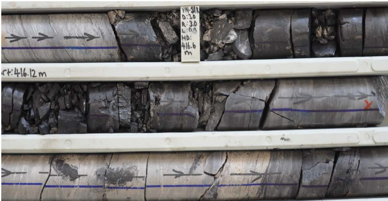
Yallourn North 1A: Core photo showing Rintouls Creek Formation comprising interbedded quartzose sandstone (reservoir: cream-white), carboniferous shale (mature source rock: dark grey-black) and black coals (mature source rock).
