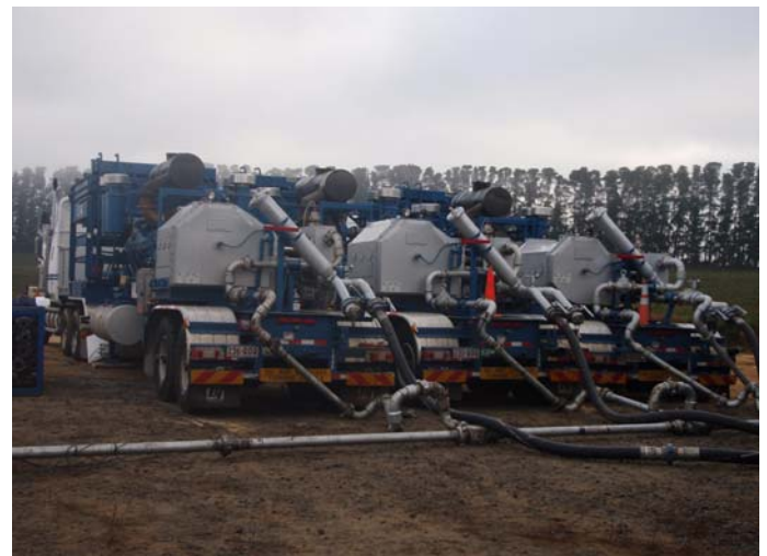
BJ frac pumping trucks on site at Wombat 2 in June 2009
