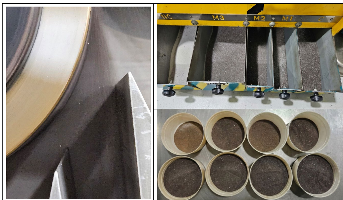
Photo 1: Rosewood RM01 material undergoing magnetic and electrostatic separation, IHC Laboratories, Brisbane. Left – Induced Roll Magnetic Separator undertaking magnetic separation to upgrade coarse concentrate. Top right – Product streams from one of the electrostatic stages. Bottom Right – Rare Earth Roll Magnet separations.
