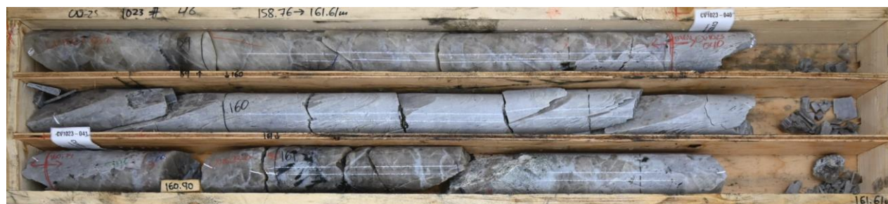
Figure 4: Massive and near-inclusion free spodumene in drill hole CV25-1023 from the Vega Zone at the CV13 Pegmatite. Core grades 1.1 m at 7.32% Li 2 O (from 159.6 m to 160.7 m) within a wider mineralized interval of 31.2 m at 2.07% Li 2 O (133.4 m to 164.6 m). At 7.32% Li 2 O, this is the second highest grade of lithium returned from an individual core sample collected to date at the Property.
