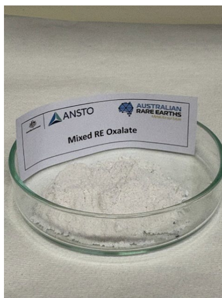
Figure 1: Sample of AR3's mixed rare earth oxalate
