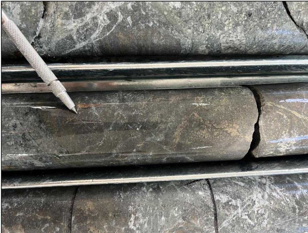
Figure 6: Core photo of polymictic breccia with pyrrhotite and chalcopyrite in ZRSD252230 from 504.5 to 506.0m - 5.9 g/t Au, 2.0% Cu & 3.6 g/t Ag (9.5 g/t AuEq 2 ).
