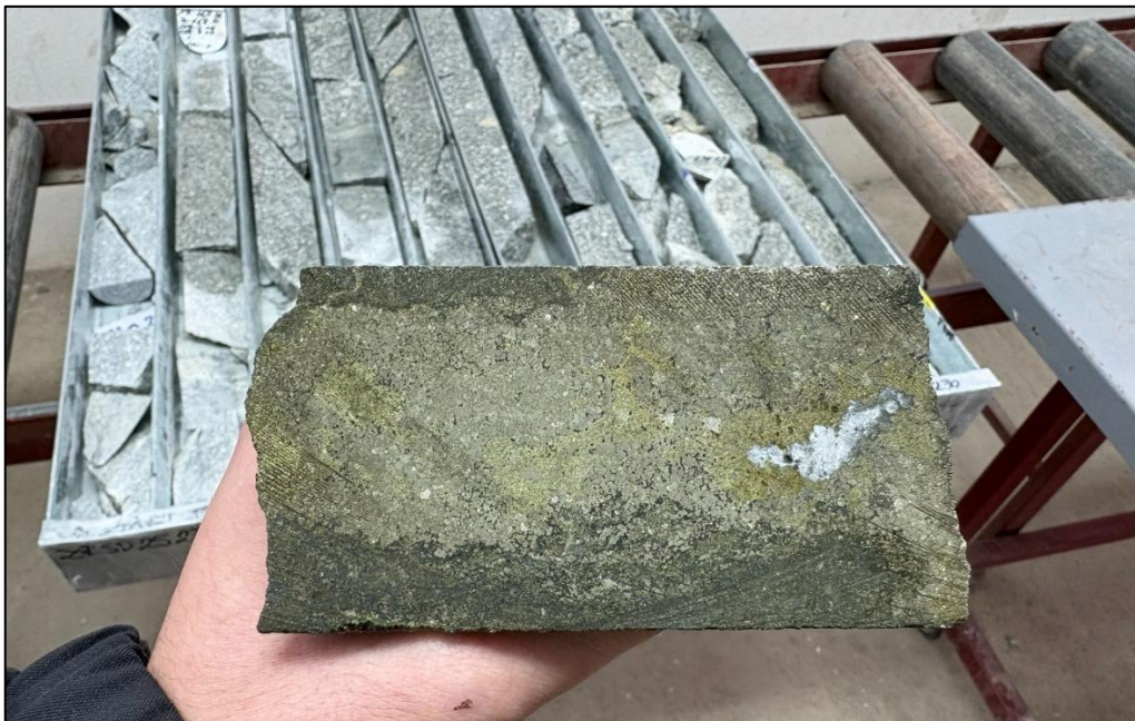
Figure 5: Core photo of massive pyrite and chalcopyrite in green garnet skarn in ZRSD25228 from 317.1 to 317.6m - 1.8g/t Au, 7.2% Cu, 0.3% Pb, 0.1% Zn and 229.0g/t Ag (18.1 g/t AuEq 2 ).
