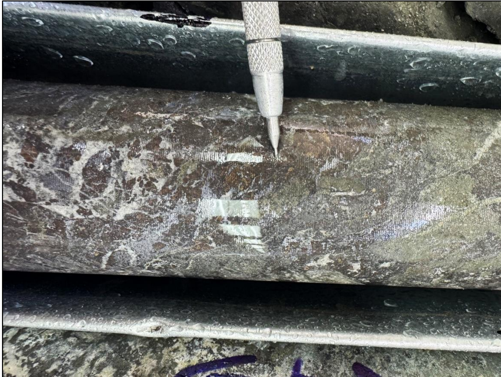
Figure 4: Core photo of massive sphalerite, galena and pyrite with minor arsenopyrite and chalcopyrite in green garnet skarn in ZRSD25222 from 533.4 to 534.7m - 0.2 g/t Au, 0.2% Cu, 20.0% Pb, 13.8% Zn & 253 g/t Ag (19.2 g/t AuEq 2 ).
