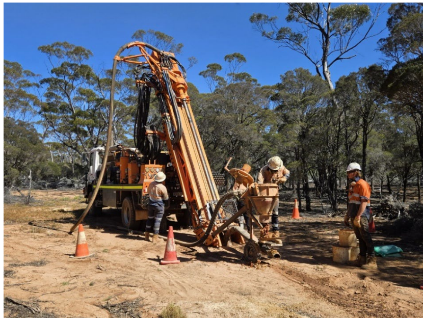
Figure 9 - Aircore drilling at Merrivale South REE prospect
