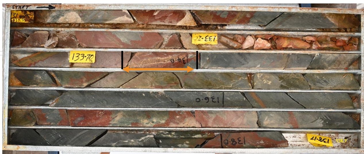
Figure 8: Mt Solitary - MS32 131.95 – 138.17m including (assay 131.95-134.0m 7.7g/t Au) hosted in crustiform veins (orange arrow) within a broad zone of increased chlorite and silica alteration and elevated iron oxides.
