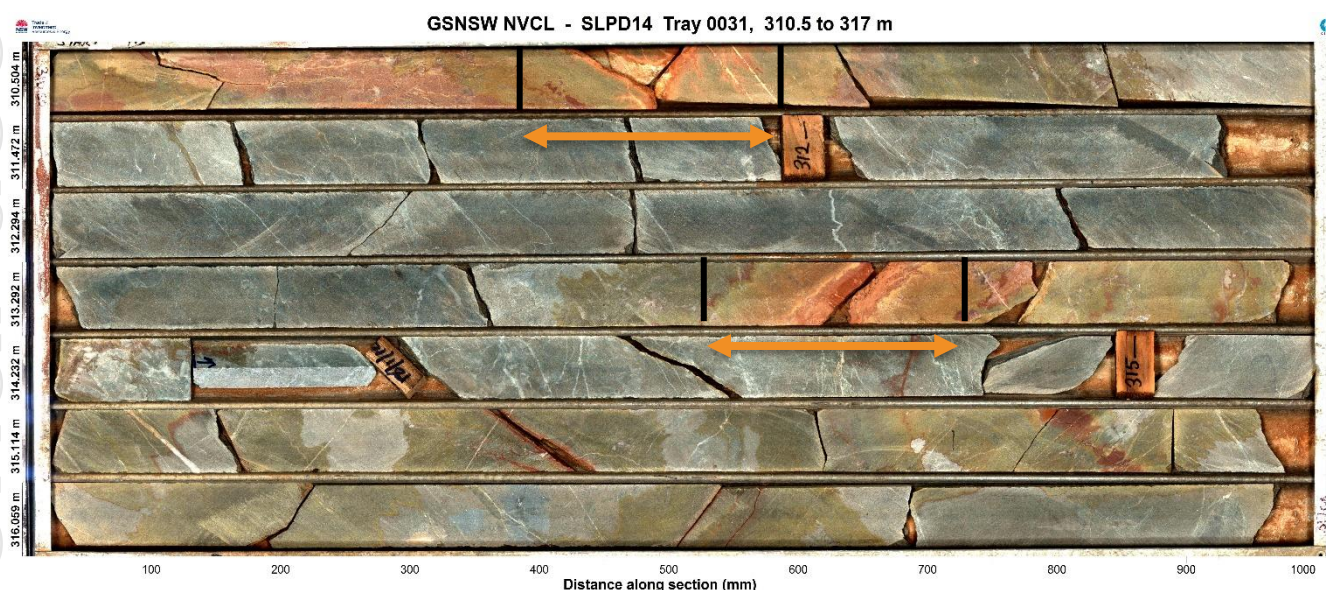
Figure 7: Mt Solar -SLPD014 8m at 1.94g/t Au (from 310-318m) in crustiform style silica flooded veins (orange arrows) with a broad zone of increased chlorite and silica alteration and elevated iron oxides.
