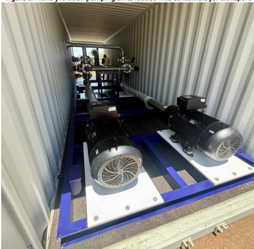
Figure 2. Nano-filtration pumping units loaded into containers for transport
