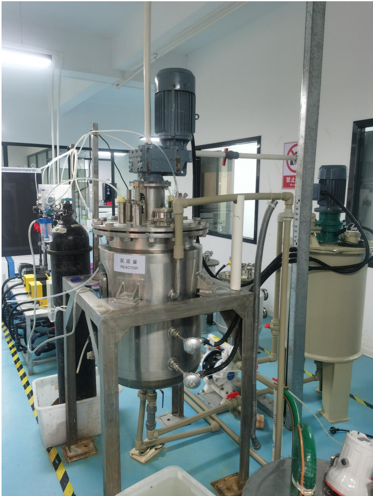
Figure 2. The Company's patented precursor MFP reactor vessel.
