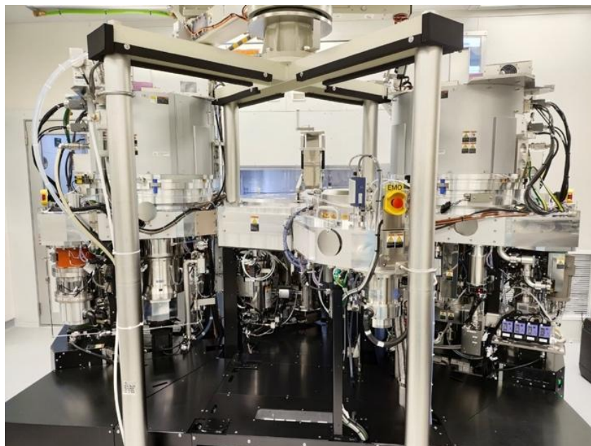
Figure 1: RRAM deposition tool used by Artemis Labs to build and refine the thin-film memory layers for DorsaVi's next-generation RRAM devices, supporting the Company's transition toward advanced 22 nm technology nodes.
