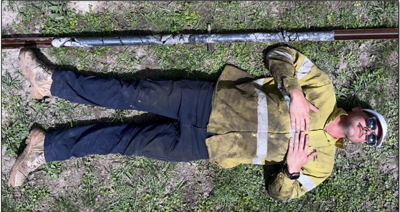
Figure 1 : DTM driller and 1.6m of the 2.2m section of CBADD010 where massive stibnite and quartz veining with stibnite was intersected. A small (20cm) fault zone is also present in this interval. *
