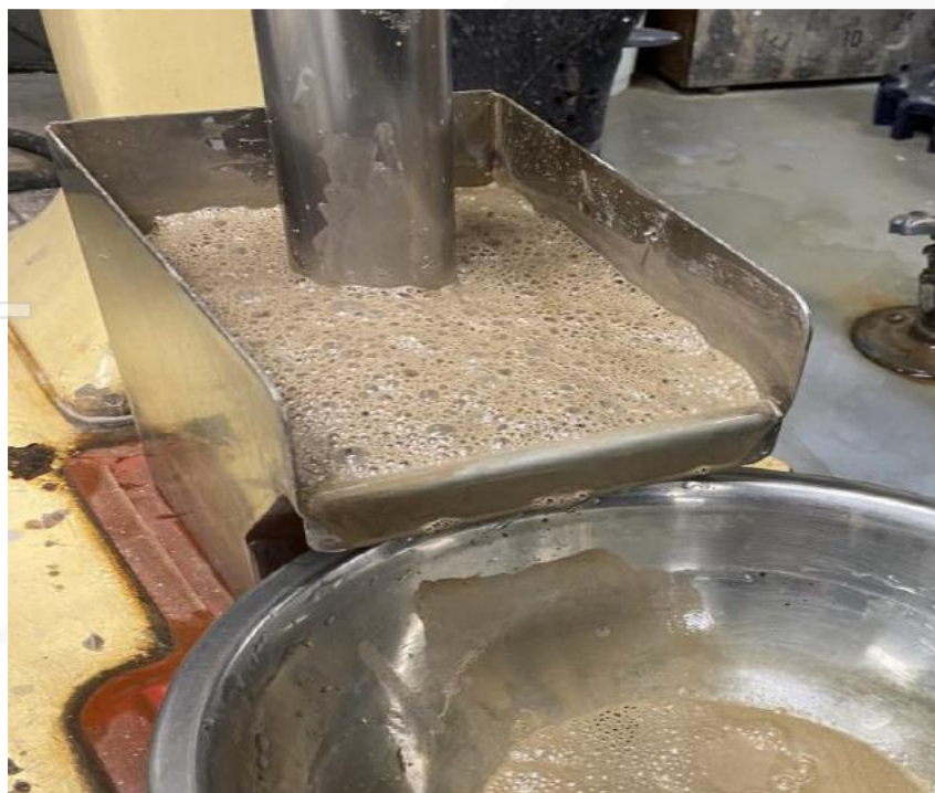
Figure 2: Flotation of Ashram whole rock sample material in a 2-litre Denver cell.
