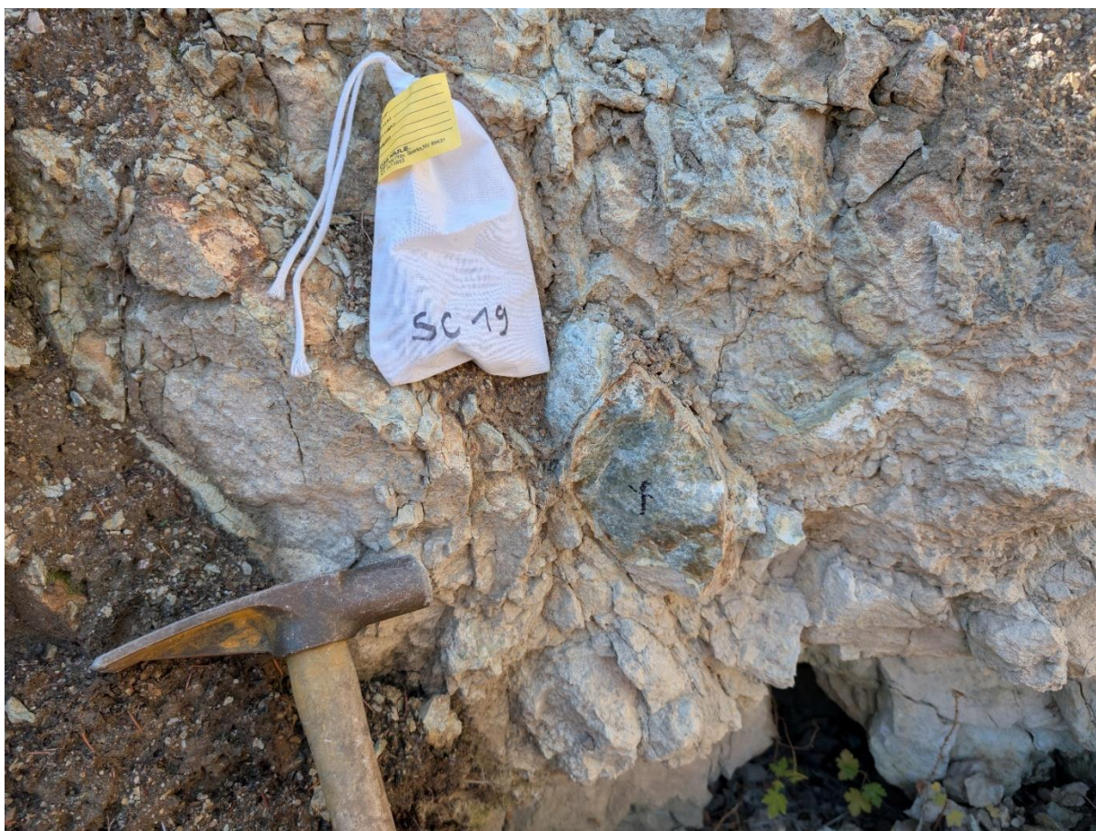
Figure 7: Photo showing outcrop of weathered silicified granite with small amounts of disseminated sulphides. Sample SC19 returned 1.1 g/t Au and 34.8 g/t Ag (see table 1 and Appendix B)
