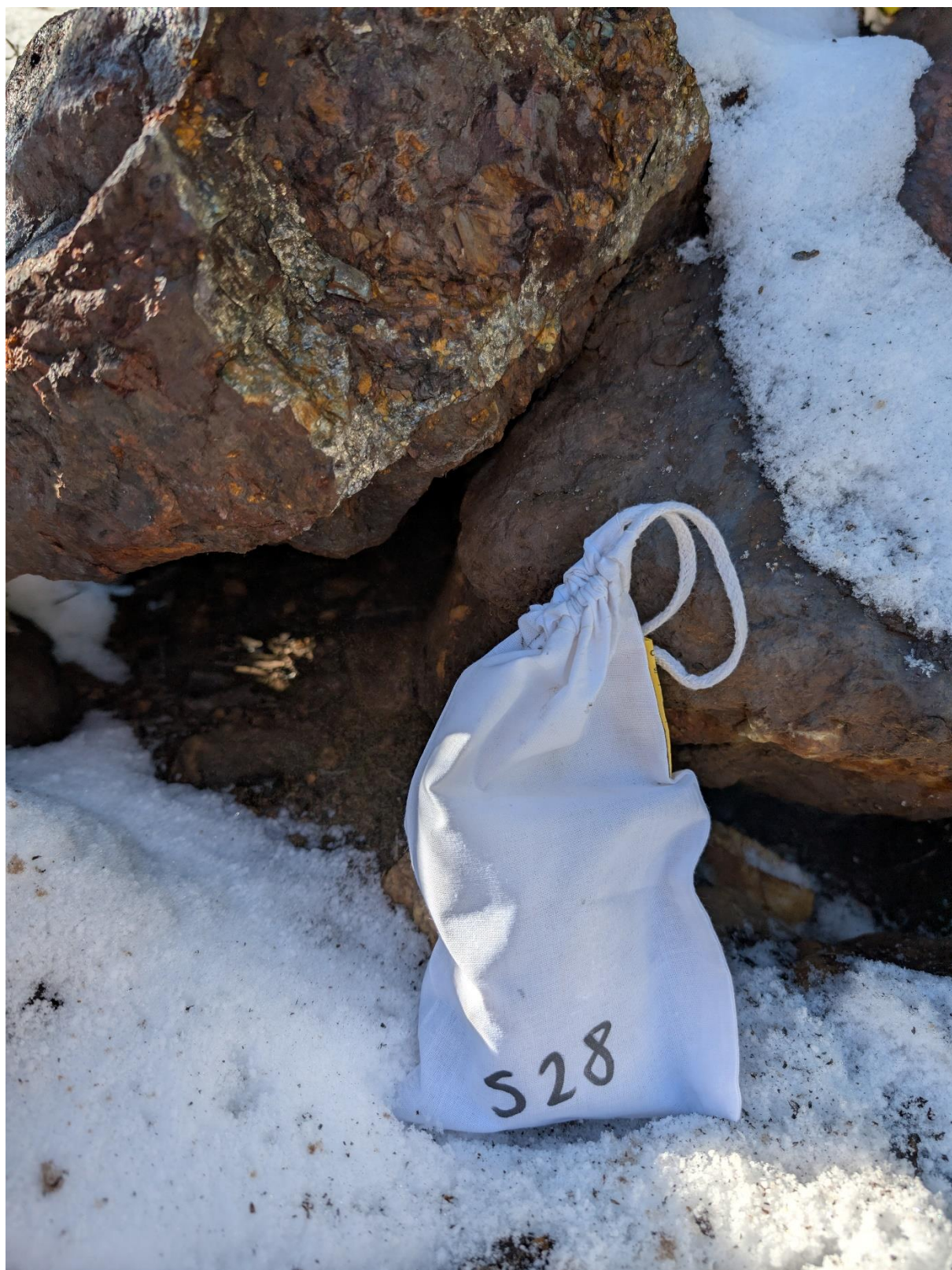
Figure 4: Picture showing sample 28 and massive pyrrhotite associated with tungsten mineralisation. Sample 28 returned tungsten grades of 0.96% (see table 1 and appendix B)
