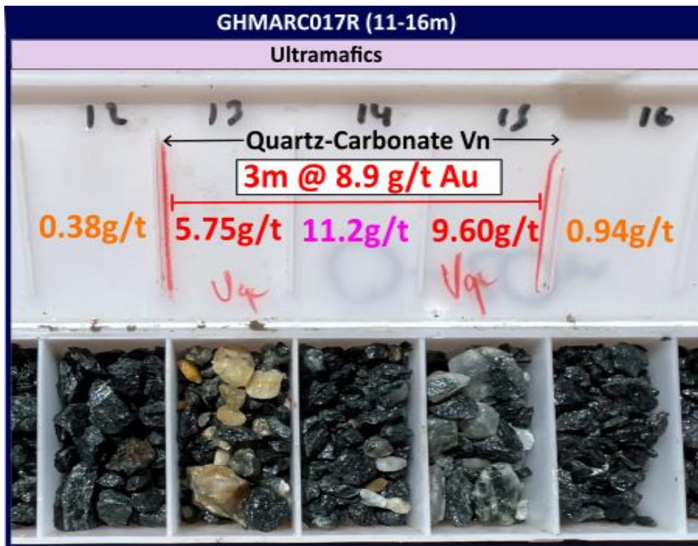
Figure 6: GHMARC017R RC chip tray showing high grade interval zone of 3m @ 8.9 g/t Au from 12m within 5m @ 5.6 g/t Au intercept in an ultramafic unit.
