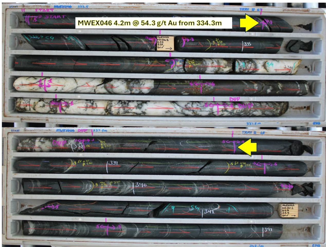
Figure 3. Example of gold lode at Mulwarrie in drill core, from MWEX046 334.3m to 338.5m; 4.2m @ 54.3 g/t Au
