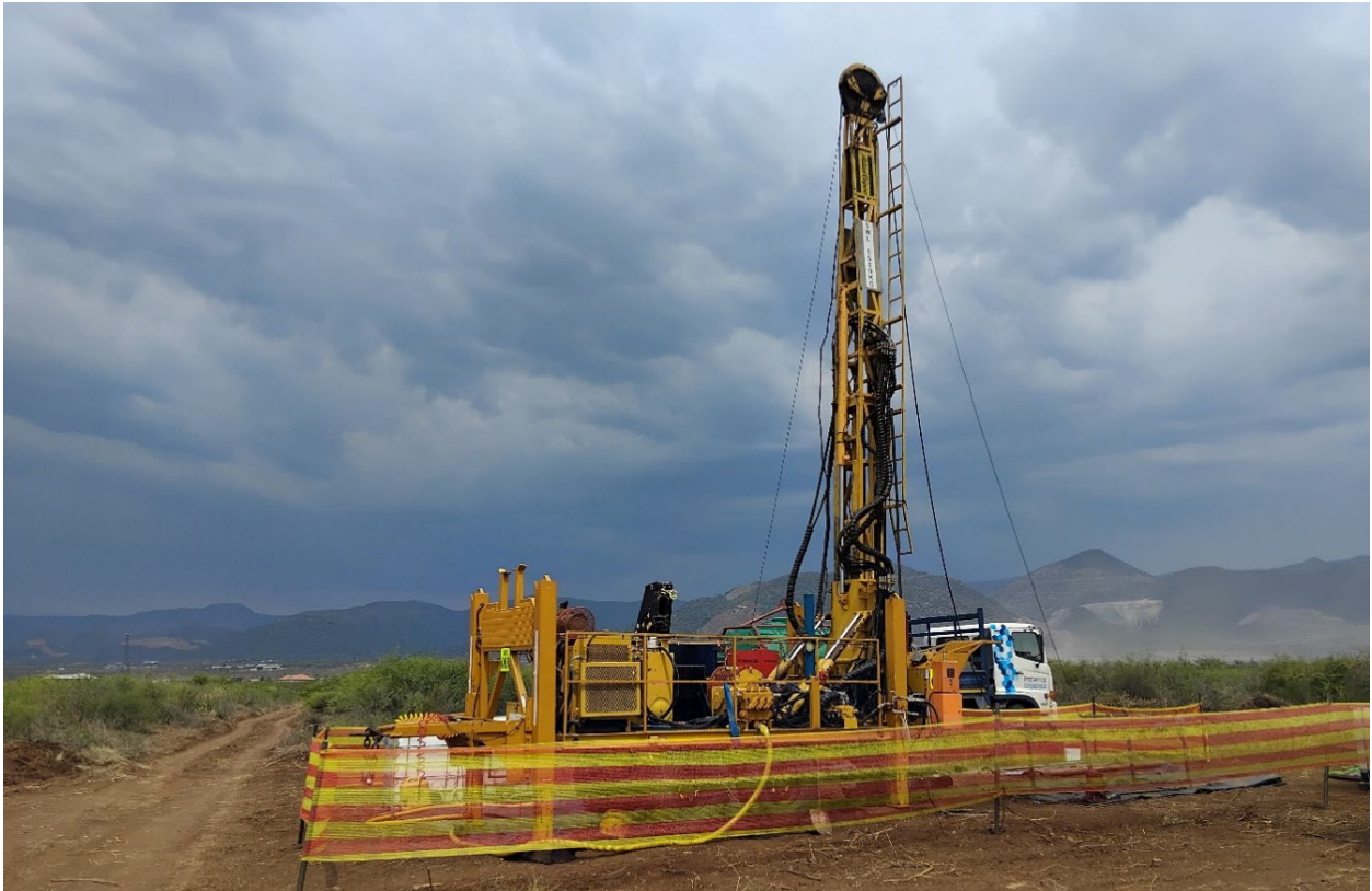
Figure 1: Atlas Copco CS1500 Drill Rig undertaking metallurgical sampling
