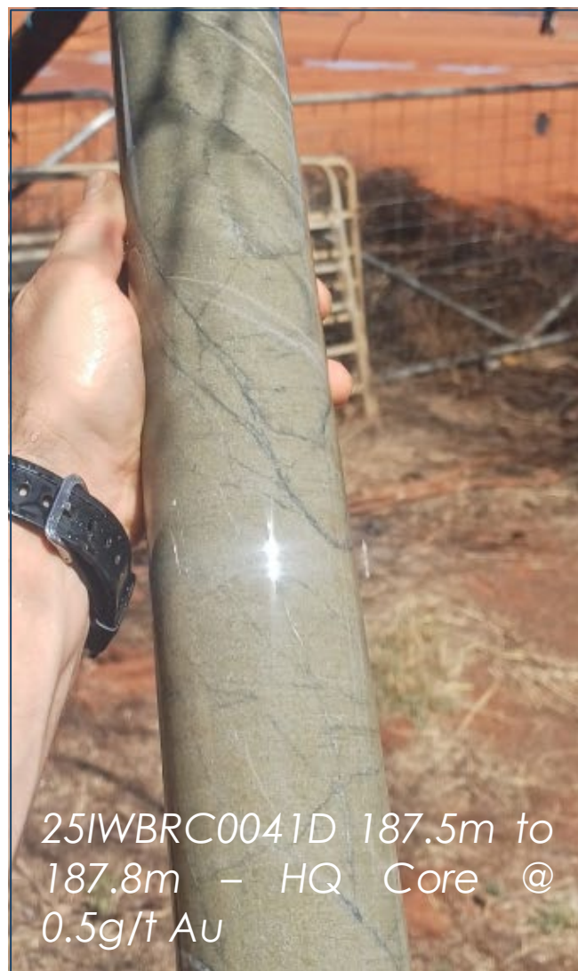
Figure 4: Example of higher-grade Arrakis mineralisation from HQ core (~63.5mm diameter core) intercepted in 25IWBRC0041D.
