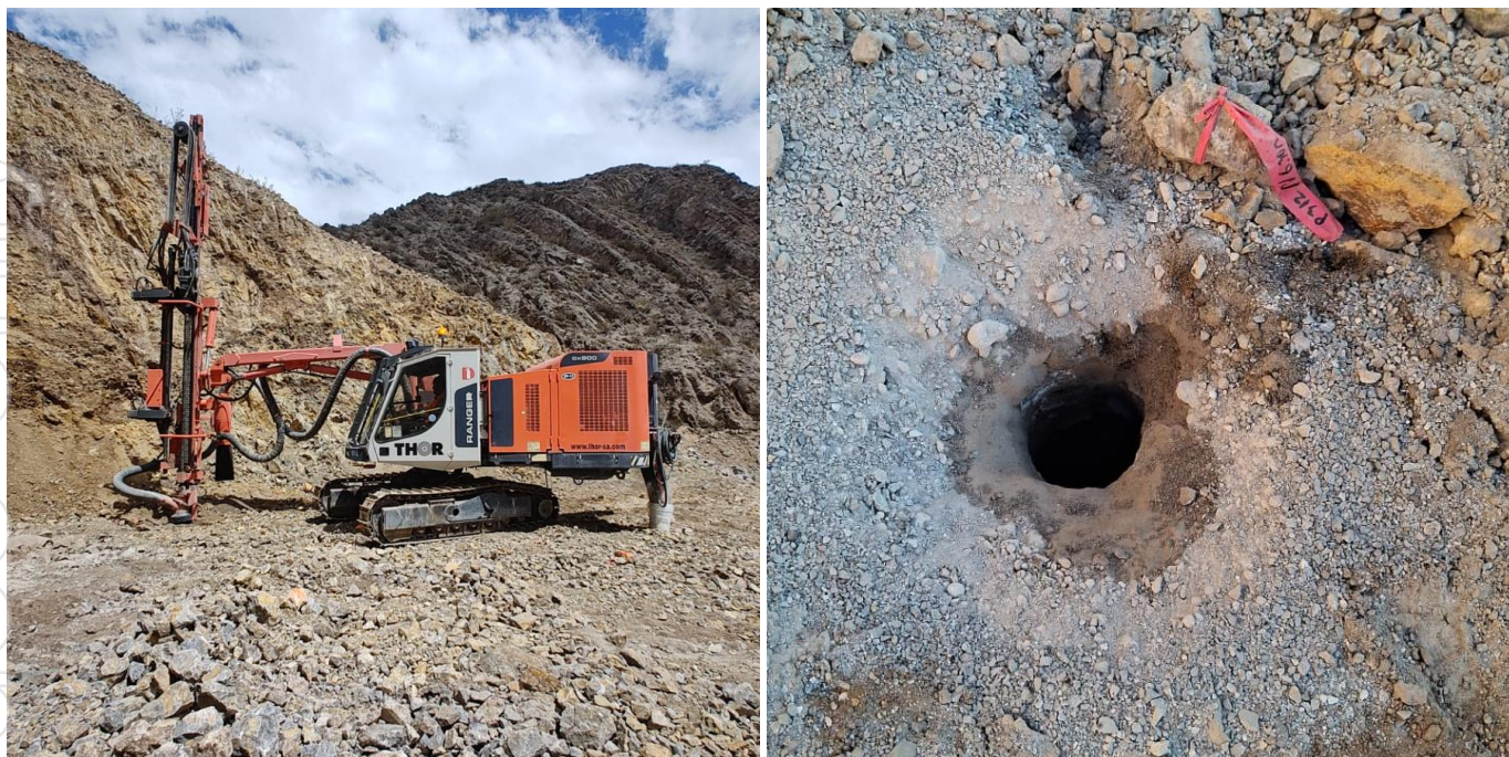
Figures 1 and 2 – THOR Blasthole Rig ready to commence drilling operations (L); and, the first production blasthole at Hualilán.
