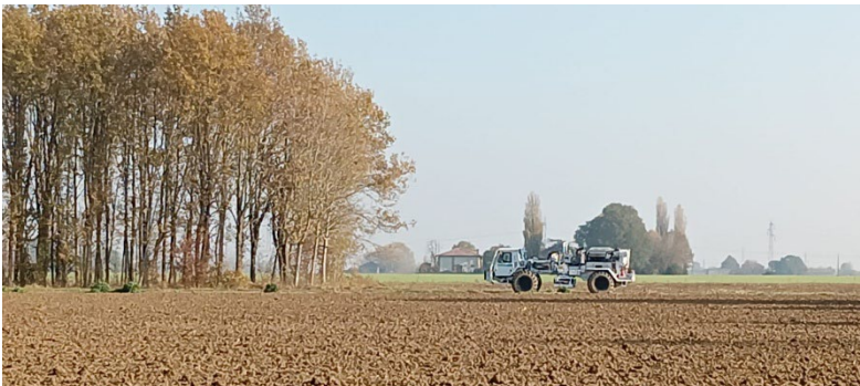
Image 5 – Vibroseis truck on field performing sweep for 3D Seismic Survey
