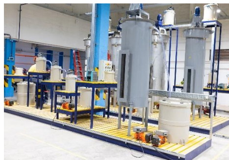
Figure 6 – Impurity Removal Circuit
