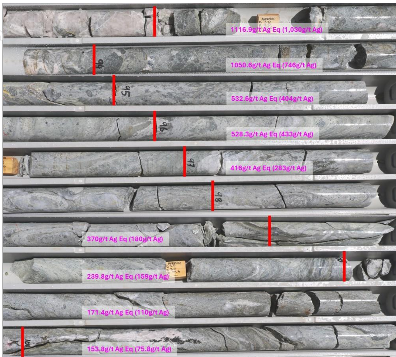
Figure 3 – Photo of Drill Core from AKDD210 showing the Ag Eq and Ag Assay Results within massive foliated baritic-greywacke
