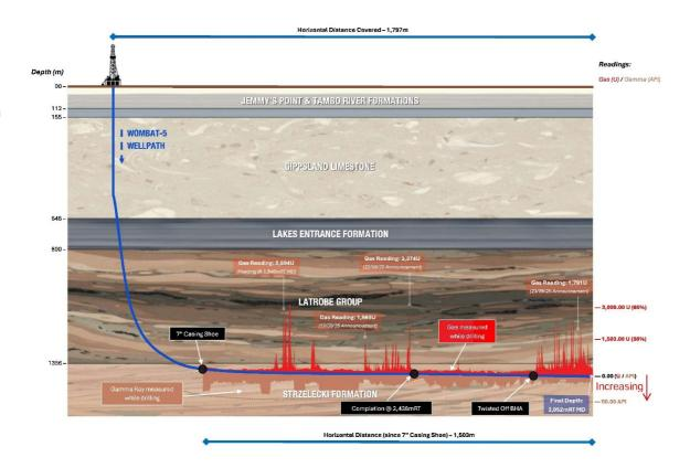
Schematic cross-section showing the Wombat-5 well path and significant gas shows to be tested during the production testing operations.
