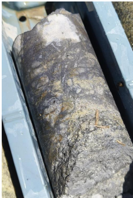
Figure 7: Breccia zone example from 171.0-171.2m in CBADD002. Sulphides are present within the breccia matrix, breccia clasts are largely quartz. Logging and sampling have been completed and the return of assays is expected in November.
