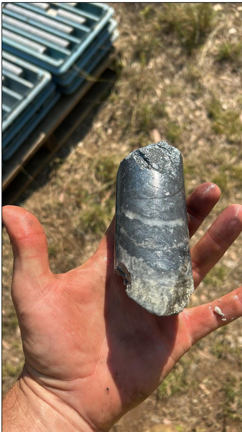
Figure 2 Stibnite and quartz veining from 42.0-42.1m downhole in Dart Mining's first drill hole at Coonambula (CBADD001). This is an example only and no sampling and assaying has been completed. Assay results have been provided in the attached ASX:DTM Announcement*.
