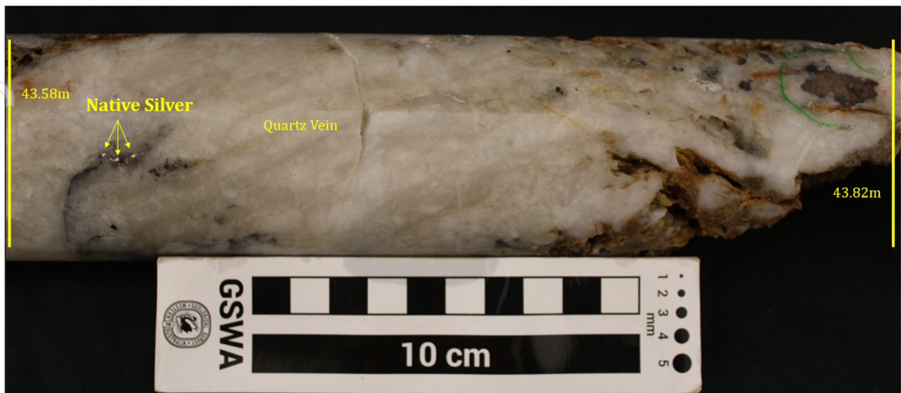
Figure 7. Photograph of HQ3 diamond drill core (25WCDD017) from 43.58m to 43.82m showing several up to 2mm wide native silver grains (<0.5%) confirmed by pXRF within a massive quartz vein.
