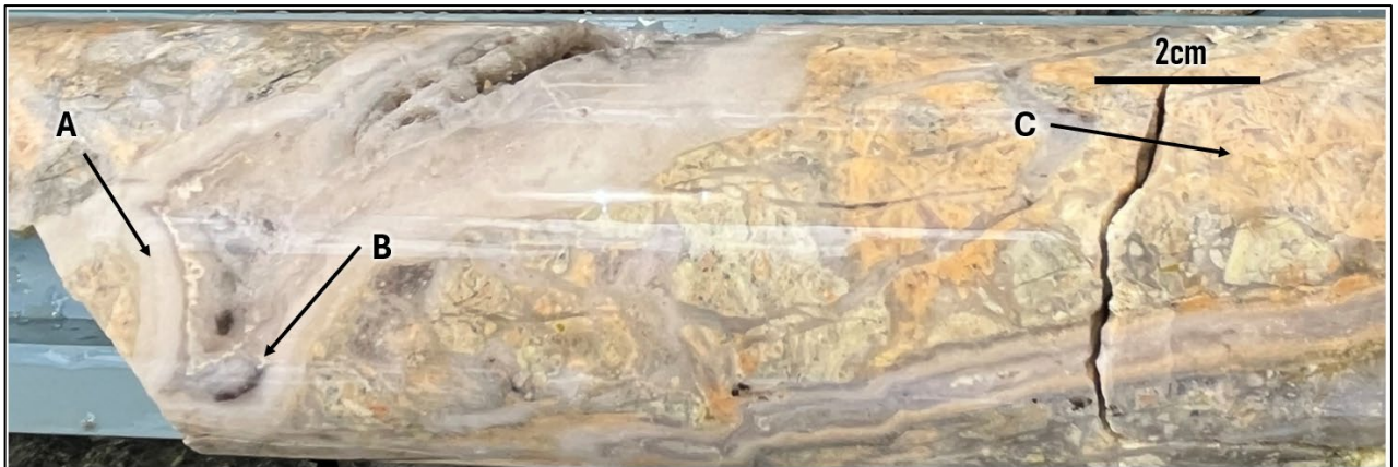
Figure 4: Cockade (A) sulphide banded (B) quartz-adularia (C) veining within the high-grade A-Vein interval reporting 2.8m @ 15.15g/t Au from 59.2m in 25FCDD010.
