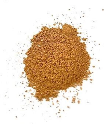
Figure 1: Initial Mixed Rare Earth Product (oxide) 84% TREO
