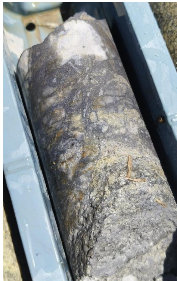
Figure 2: Breccia zone example from 171.0-171.2m in CBADD002. Sulphides are present within the breccia matrix, breccia clasts are largely quartz. Logging and sampling have been completed and the return of assays is expected in November.
