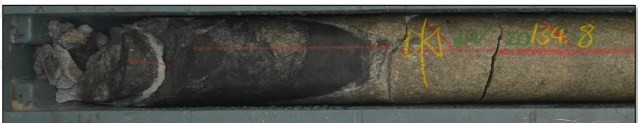
Figure 3: Massive Stibnite from CBADD002 showing massive stibnite Vein between 134.5 to 134.8 with estimated 80% Stibnite. Assays expected in November.
