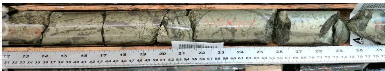
Figure 2: Spectacular 'bonanza grade' intersection of massive chalcopyrite-pyrrhotite mineralisation, 0.5m @ 22% Cu, 0.78% Ni, 11g/t Pd, 3.6 g/t Pt, 0.24 g/t Au from 55.3m (19-ZA-05). Forms part of 15.7m @ 3.1% Cu, 1.6% Ni, 2.2 g/t Pd, 0.6 g/t Pt, 0.25 g/t Au. Drilled by Chase Mining in 2019.
