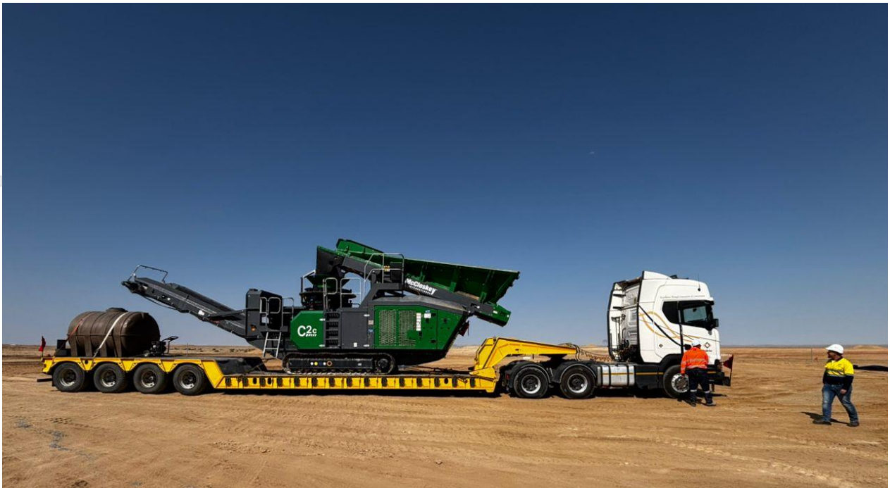
Figure 3: The first crusher has arrived onsite at Etango for the crushing of aggregate for the heap leach drainage layer.
