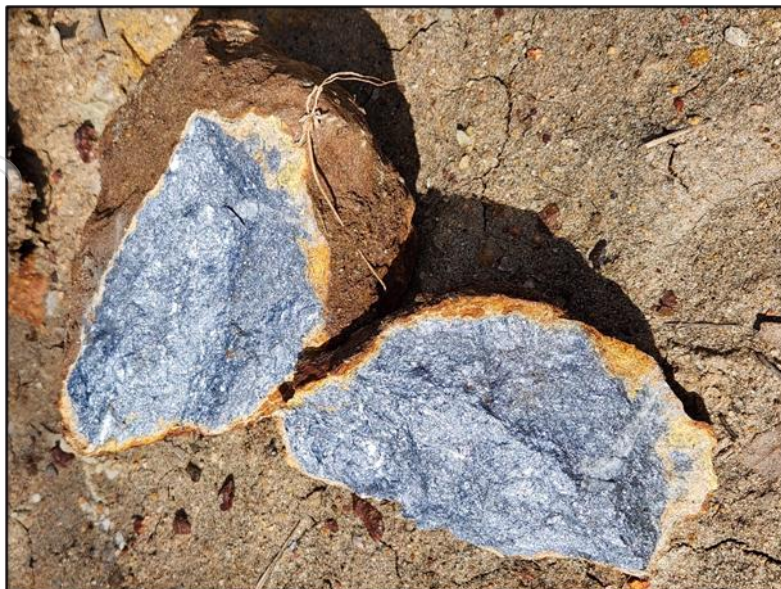
Figure 1 Massive Stibnite from sample BSE04 returning 55.5% Sb
