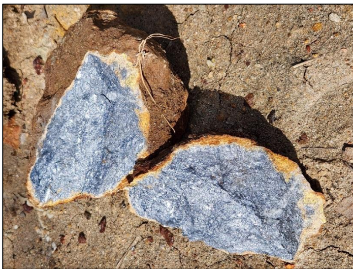
Figure 1: Massive Stibnite from sample BSE04 returning 55.5% Sb
