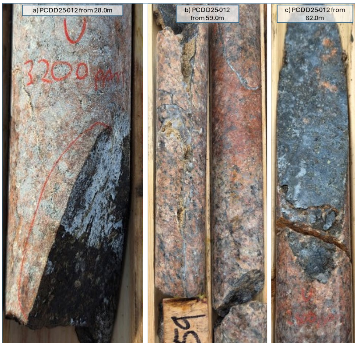
Figure 2: Drill core from PCDD25-012 (470459E, 5557965N, UTM Zone 21) with significant uranium mineralisation detected using pXRF.
