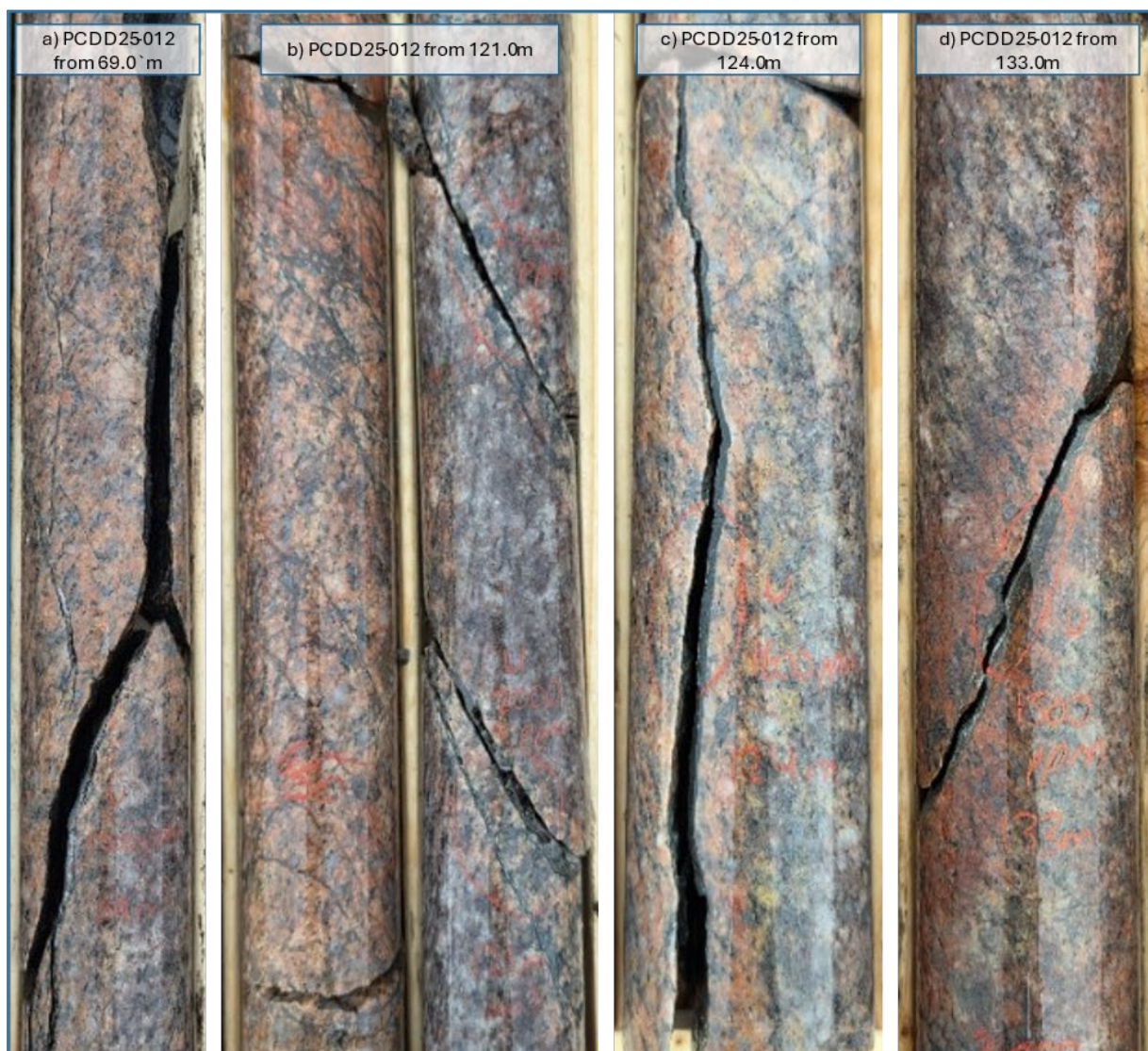
Figure 3: Drill core from PCDD25-012 (470459E, 5557965N, UTM Zone 21) with significant uranium mineralisation detected using pXRF. Notice the variation in the type and amount of alteration of the granite that can be seen in these core samples.
