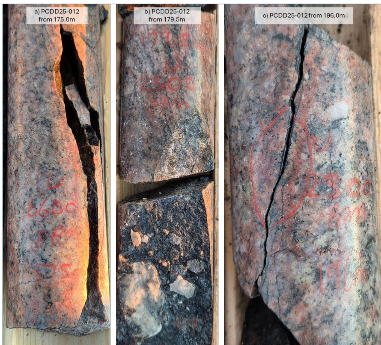
Figure 4: Drill core from PCDD25-012 (470459E, 5557965N, UTM Zone 21) with significant uranium mineralisation detected using pXRF.
