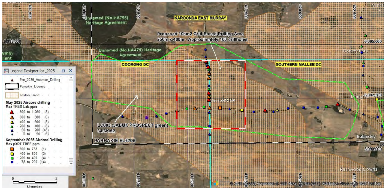
Figure 3: Jabuk Prospect showing the most recent (September 2025) road verge drilling, significant TREE intervals and proposed close spaced grid drilling area (broken red line boundary).
