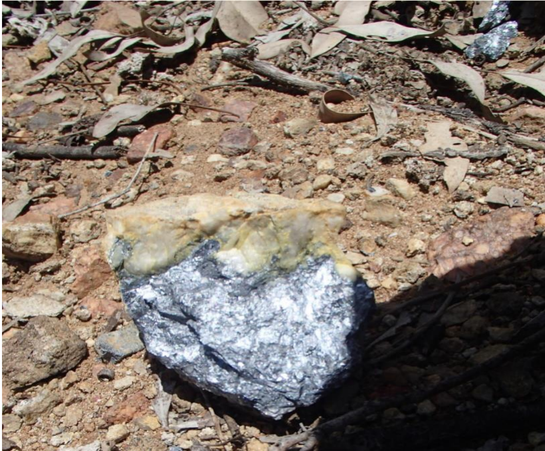
Figure 4 - Banshee mine waste dump material observed (unsampled) by Dart Mining in January 2025 showing antimony mineral (70% stibnite*) with encasing vein quartz
