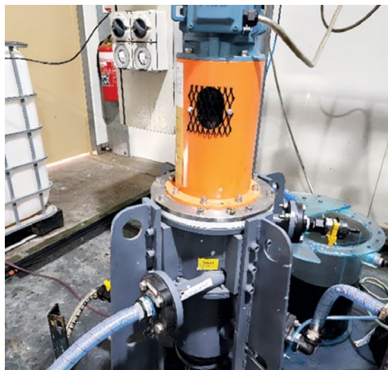
Figure 3 – Electrowinning cells used for testing (LHS) and Centrifugal extractor (RHS)
